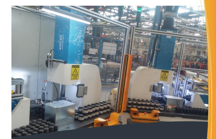
Lower Arm Rubber Bushing Inserting
